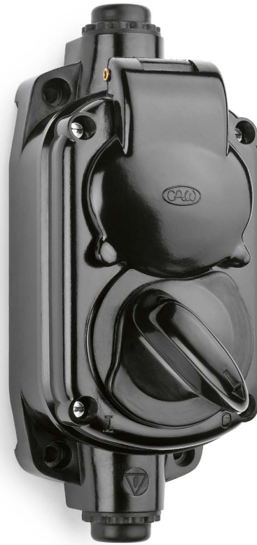
Garage outlet surface-mounted 2-pin. 16 A, AC 250 V, IP20. 70 x 170 mm, Height above surface 87 mm. Case and lid made of Bakelite®. With screw contacts. Product code 100295
