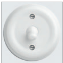
SURFACE-MOUNTED TOGGLE SWITCH DUROPLAST 10 A, 10 AX, AC 250 V, IP 20 62 mm Ø, height above surface incl. toggle 49 mm. Duroplast housing and toggle.
