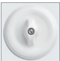
SURFACE-MOUNTED ROTARY SWITCH DUROPLAST 10 A, 10 AX, AC 250 V, IP 20 62 mm Ø, height above surface incl. locking bolt 53 mm. Duroplast housing and locking bolt. With spring clip.
