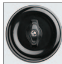
SURFACE-MOUNTED ROTARY SWITCH BAKELITE 10 A, 10 AX, AC 250 V, IP 20 62 mm Ø, height above surface incl. locking bolt 53 mm. Bakelite housing and locking bolt. With spring clip.
