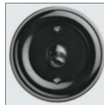
SURFACE-MOUNTED TOGGLE SWITCH BAKELITE 10 A, 10 AX, 250 V, IP 20 62 mm Ø, height above surface incl. toggle 49 mm. Bakelite housing and toggle.
