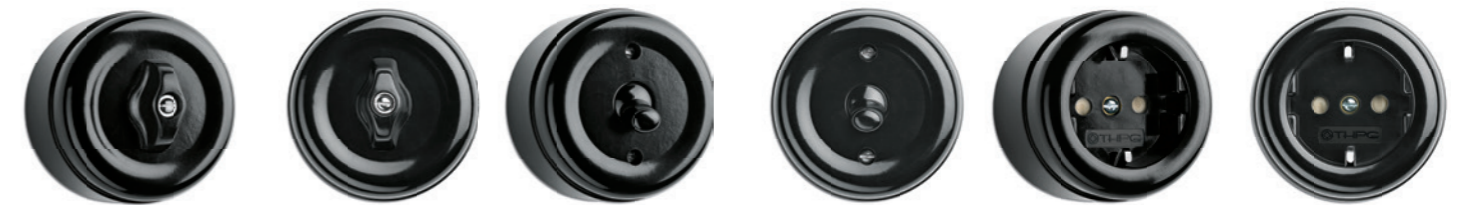
SURFACE-MOUNTED ROTARY SWITCH BAKELITE® 10 A, 10 AX, AC 250 V, IP20 62 mm Ø, height above surface incl. locking bolt 53 mm. Bakelite® housing and locking bolt. With spring clip SURFACE-MOUNTED TOGGLE SWITCH BAKELITE® 10 A, 10 AX, 250 V, IP20 62 mm Ø, height above surface incl. toggle 49 mm. Bakelite® housing and toggle SURFACE-MOUNTED OUTLET BAKELITE® 16 A, AC 250 V, IP20 62 mm Ø, height above surface 49 mm. Bakelite® housing with shutter. With spring clips. Alternation switch Crossbar switch Multi-circuit switch Order no. 186892 Order no. 186893 Order no. 186891 Order no. 184198 Order no. 184207 OUTLET WITH MIDDLE-SAFETY CONTACT BAKELITE® With shutter (French version). Order no. 100063 BASE PLATE BAKELITE® 62 mm Ø Order no. 184619
