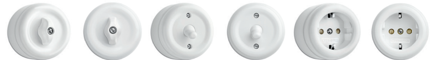
SURFACE-MOUNTED ROTARY SWITCH DUROPLAST 10 A, 10 AX, AC 250 V, IP20 62 mm Ø, height above surface incl. locking bolt 53 mm. Duroplast housing and locking bolt. With spring clip. SURFACE-MOUNTED TOGGLE SWITCH DUROPLAST 10 A, 10 AX, AC 250 V, IP20 62 mm Ø, height above surface incl. toggle 49 mm. Duroplast housing and toggle. SURFACE-MOUNTED OUTLET DUROPLAST 16 A, AC 250 V, IP20 62 mm Ø, height above surface 49 mm. Duroplast housing with shutter. With spring clips. Alternation switch Crossbar switch Multi-circuit switch Order no. 186889 Order no. 186890 Order no. 186888 Order no. 184197 Order no. 184206 OUTLET WITH MIDDLE-SAFETY CONTACT DUROPLAST With shutter (French version). Order no. 100062 BASE PLATE DUROPLAST 62 mm Ø Order no. 184642
