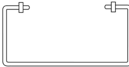
Additional items such as coverings are superfluous. A single ring or double rings offer either fixated or movable suspension. For fixated suspension, the pieces include an additional hole and an internal hexagon grub screw. The series is decorated with the red dot award.
